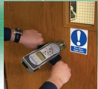
testing force to open fire door
