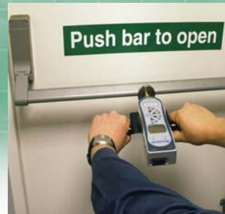
testing release force of safety bar
