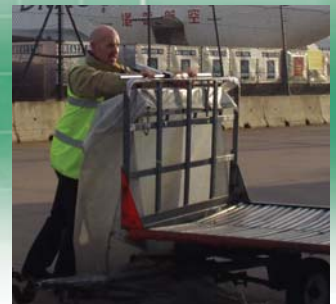
testing force to push cargo dolly
