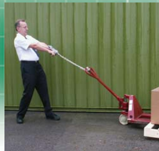
testing force to pull loaded trolley
