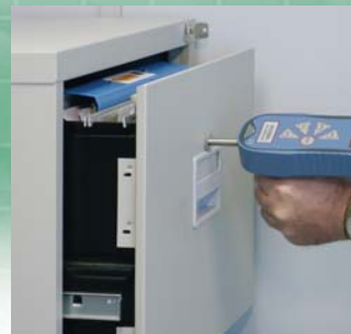
testing force to close cabinet drawer
